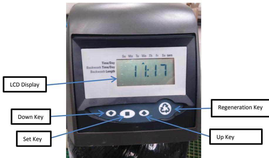
Figure 22: Key Pad and LCD Display
