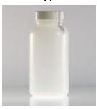
This 1,000mL sterilized bottle is used for the collection of lead and copper samples. **Lead and Copper** in water is usually caused by the corrosion of plumbing or equipment. Therefore, the best sample for detection is a "first draw" sample, or a sample taken immediately after the water has been sitting in the plumbing for at least six hours. Collecting 1,000mL of the "first draw" increases the chances of detecting Lead and Copper if it is from the plumbing.
