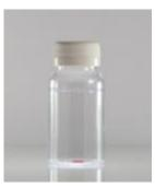
This 120mL sterilized bottle is a general purpose container most often used for **Nitrate and Arsenic**. TGA labs can perform multiple tests (including Nitrate and Arsenic) from a single bottle. Generally, use this bottle for testing anything other than Bacteria, Lead, Copper, VOC's, or Pesticides.
