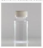
This 120mL bottle is specifically designed for the collection of water samples for **coliform bacteria**. This bottle includes sodium thiolsulfate (either in a white pill form or powder) which deactivates chlorine up to 5ppm helping to ensure the survival of bacteria from sampling to testing. This bottle should only be filled to the 100mL line.
