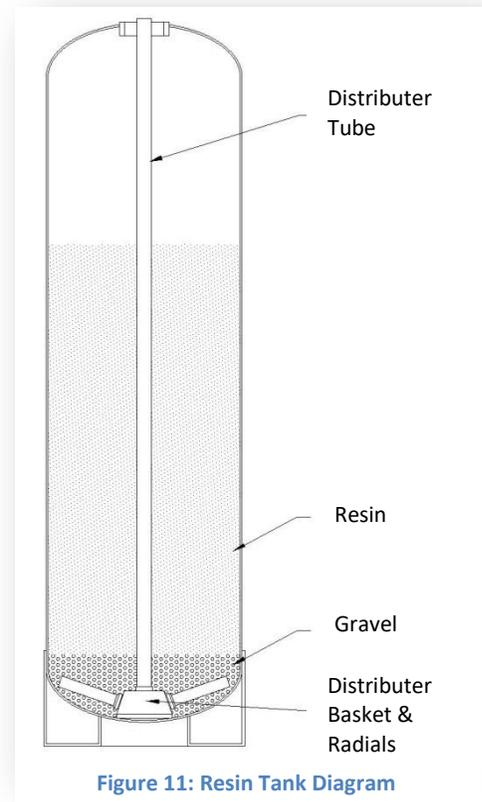
Figure 11: Resin Tank Diagram
