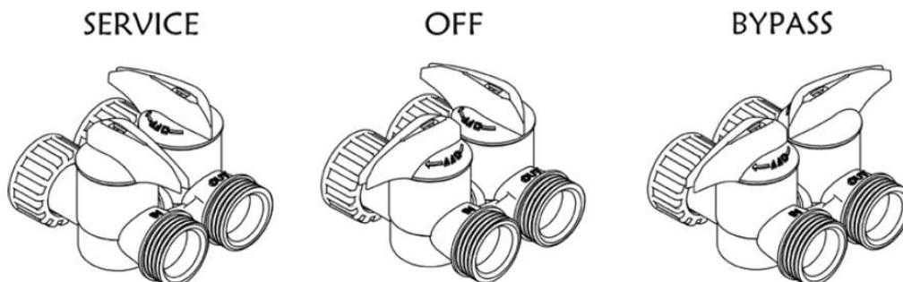
Figure 16: Bypass Valve Positions
