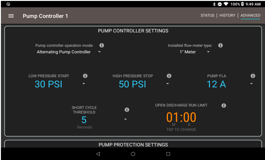
DEVICES > PUMP CONTROLLER > ADVANCED (Navigation description examples can be found in the User Guide)
