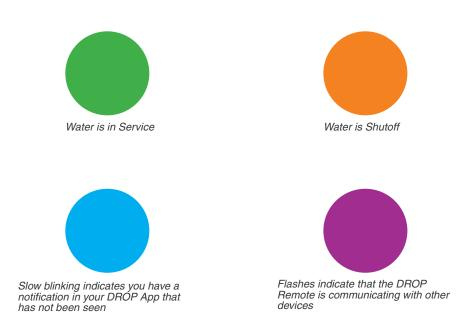
To turn off water in your home, place your finger on the water DROPlet button for about 2 seconds. Once the lights turn orange, remove your finger.
