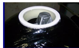
Figure 8: How to Block Distributer Tube
