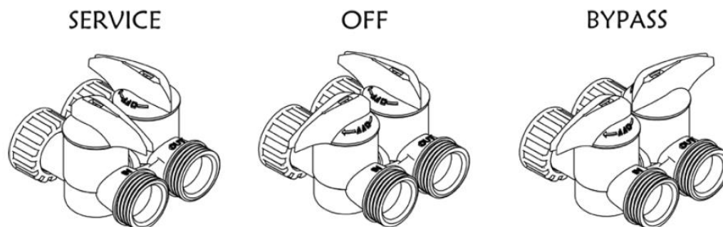
Figure 16: Bypass Valve Positions
