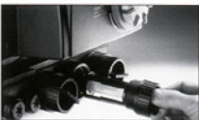
**Superior flow rate and pressure drop performance** are provided by DCS1's unique face seal diaphragm valve cartridge assemblies, manifold design and full flow path characteristics.
